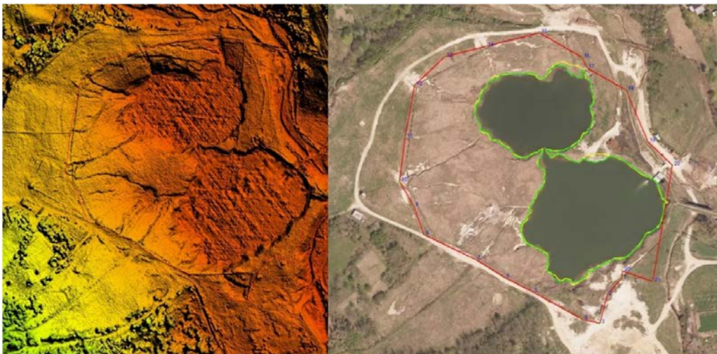
Fig. 3. The Digital Terrain Model, the orthophotomap and the control points (yellow contour - 2013, green contour-2015)
