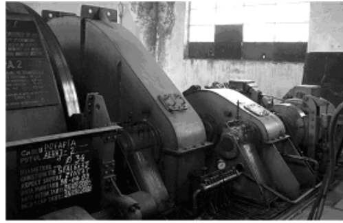
Fig. 6. Two gears reducer with separate cases
